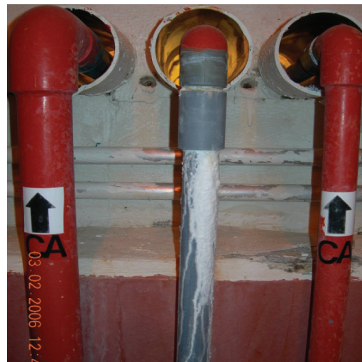
Failed solvent cement joint 25% caustic soda service.
